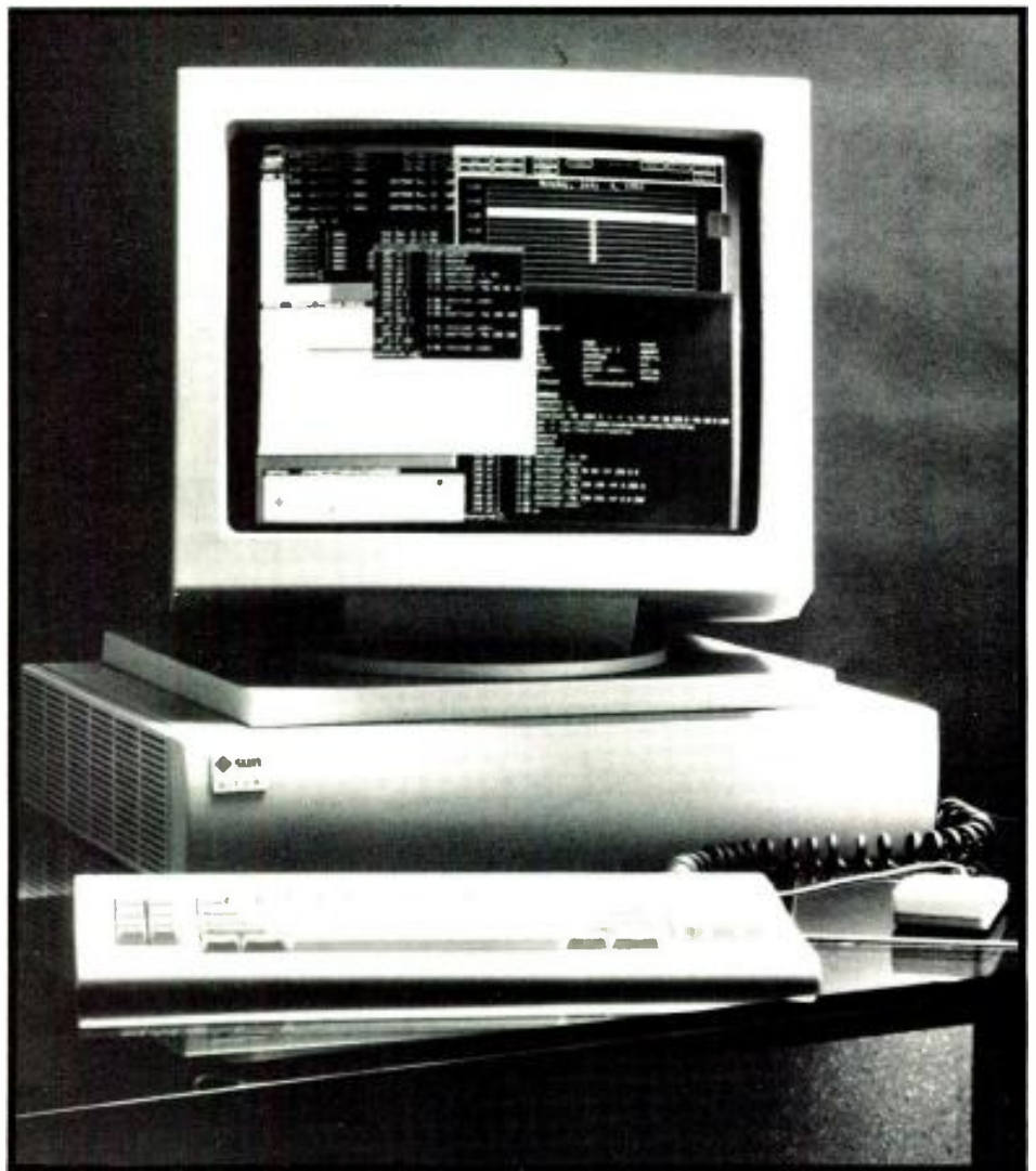
Billed by the company as the first supercomputing workstation, the Sun Microsystems 9/110 contains single in-line memory modules and a floating point processor.
